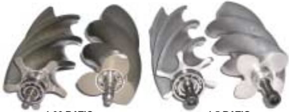
1.66 RATIO 5 X 3 ROTORS 2.3L LYSHOLM
