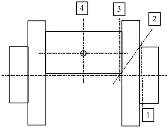
Figure 7. Critical sections for fatigue resistance
