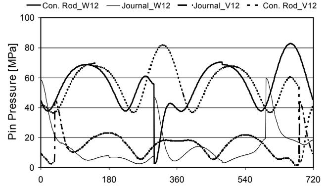
Figure 9. Pressure on the crankpin and journal against crank angle
