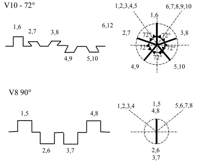
Figure 11. Sketch of the V10 and V8 crankshaft
