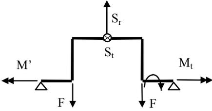
Figure 5. Sketch of the crank model and loading
