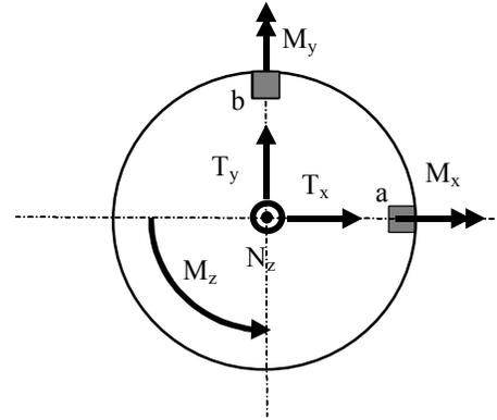
Figure 8. Load on a pin section: bending moments ( $M_x, M_y$ ), torque moment ( $M_z$ ), normal force ( $N_z$ ), shear forces ( $T_x, T_y$ )
