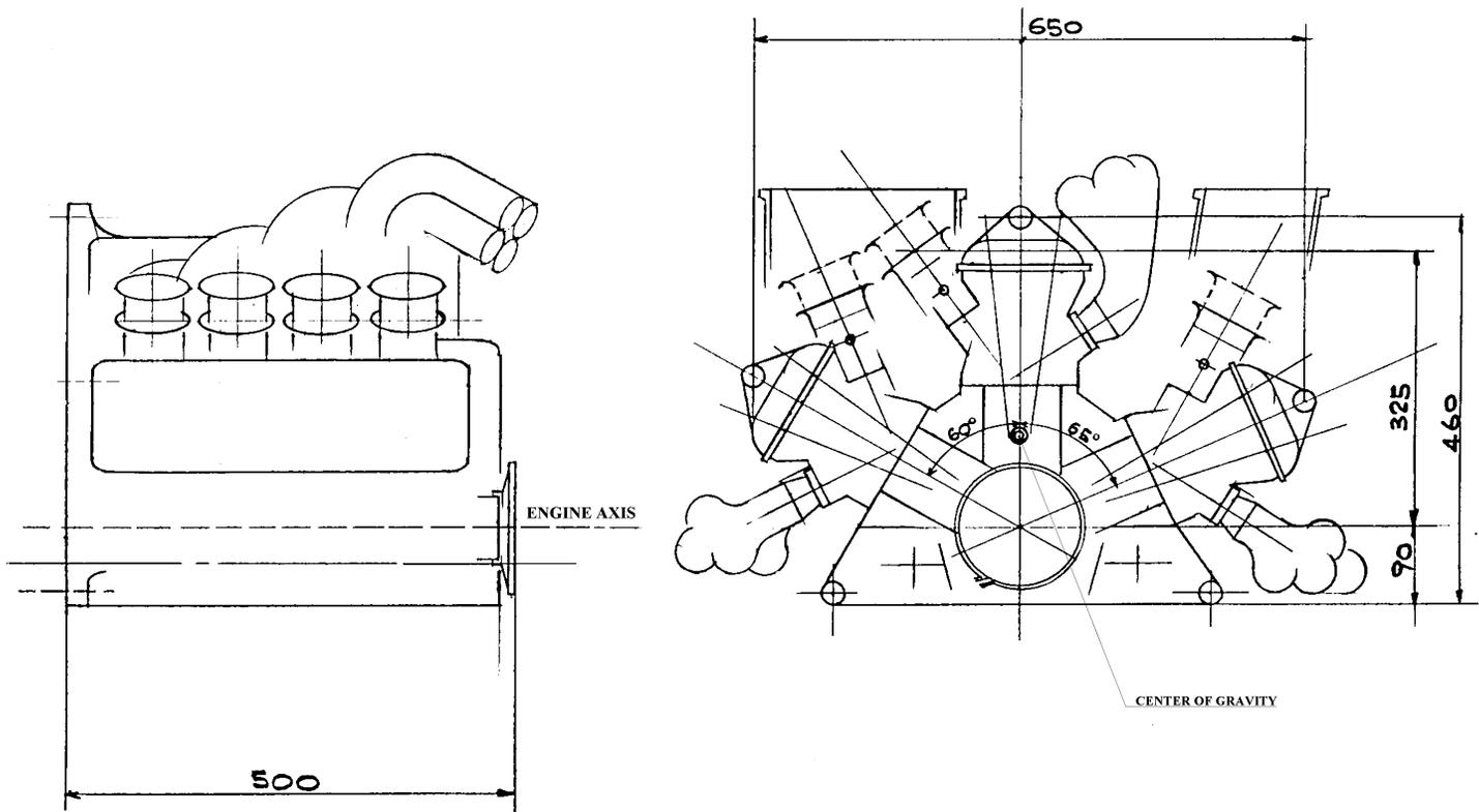
Figure 1. Lay-out of the W12 engine. It is made up of three banks of cylinders and one simple crankshaft. Each crankpin bears three equal connecting rods, one from each bank. The engine is connected to the cockpit by 5 point.
