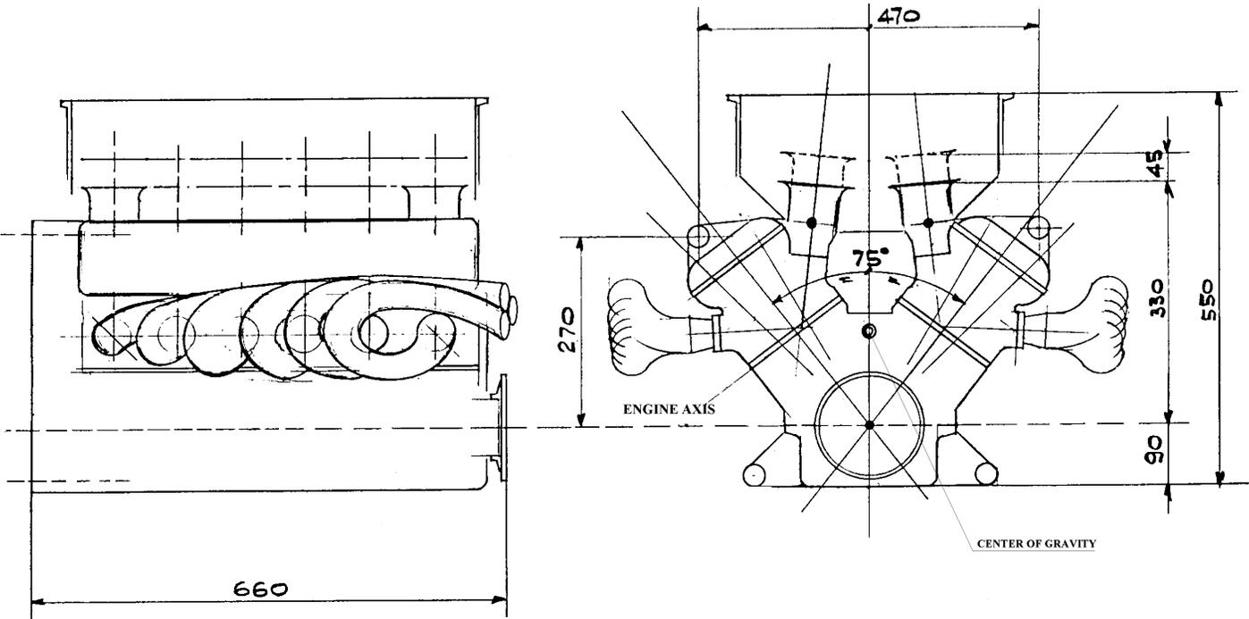
Figure 2. Lay-out of a traditional V12 engine. The engine is connected to the cockpit by 4 points.
