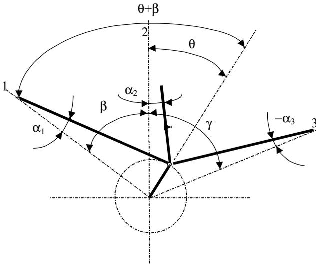
Figure 6. Sketch of the crank with the connecting rods
