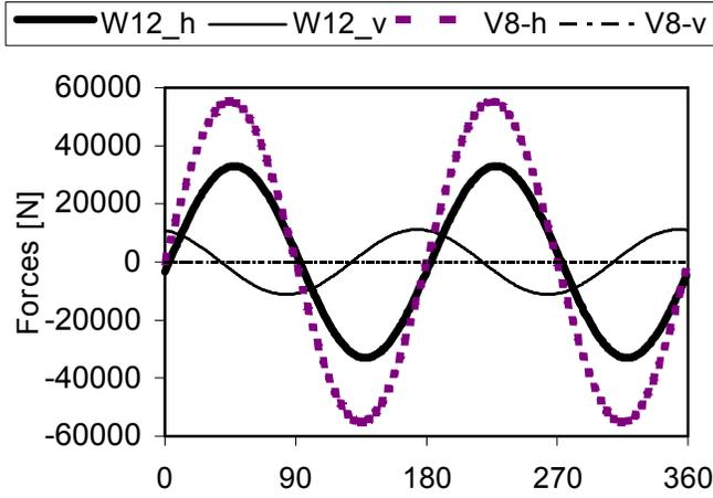
Figure 12. Unbalanced crankshaft forces.
