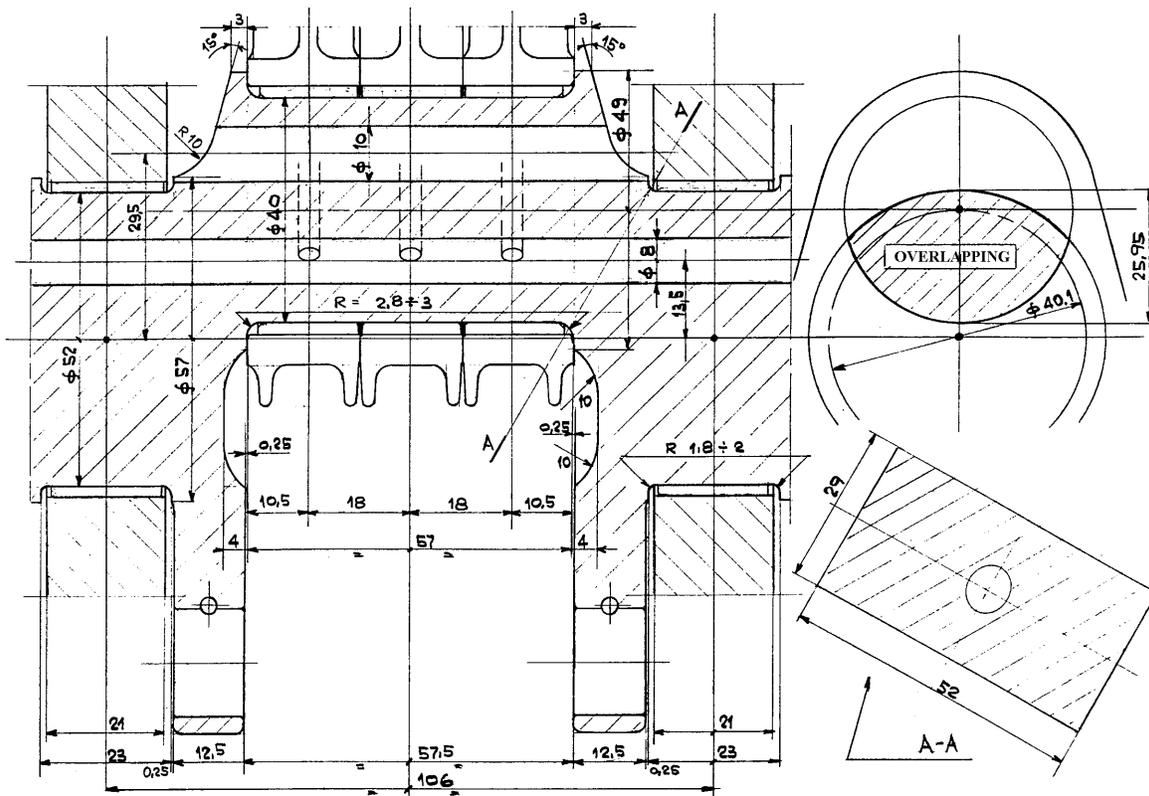
Figure 4. Working drawing of one W12 crank.
