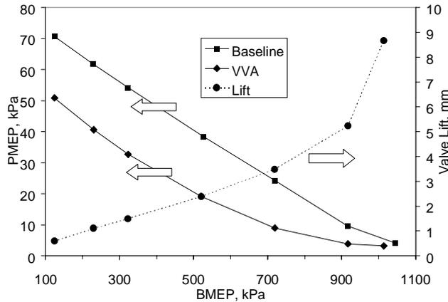
Figure 16. PMEP v. BMEP at 2000 rpm
