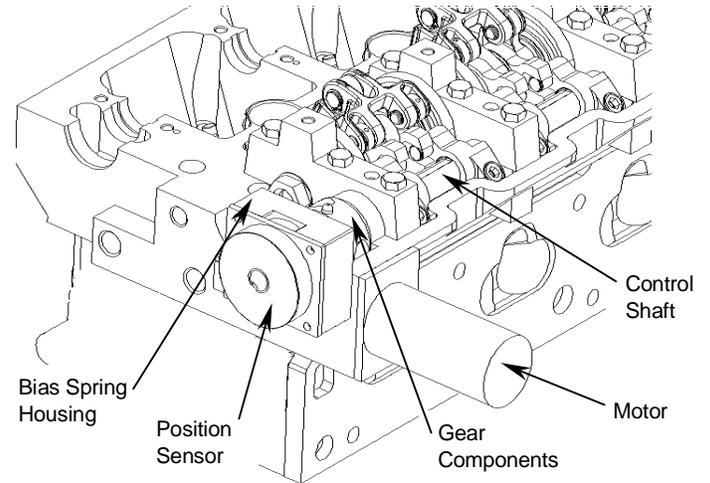
Figure 4. Actuator installed in cylinder head
