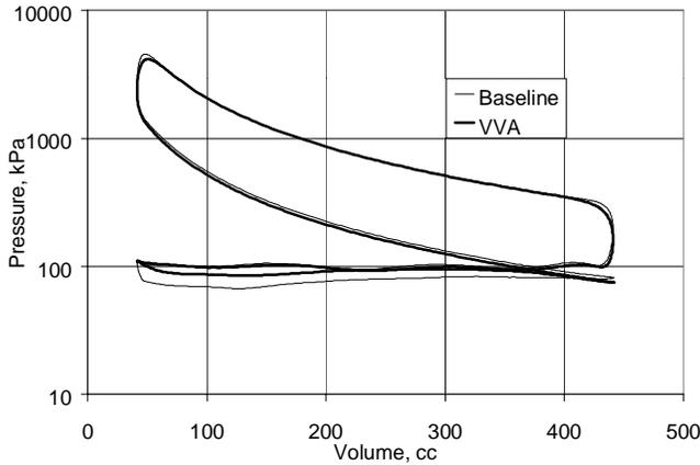
Figure 11. Pressure v. Volume: 2000 rpm / 800 kPa NMEP
