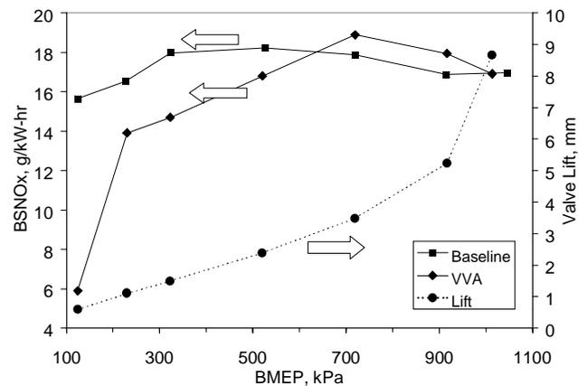
Figure 20. BS NO<sub>x</sub> v. BMEP at 2000 rpm
