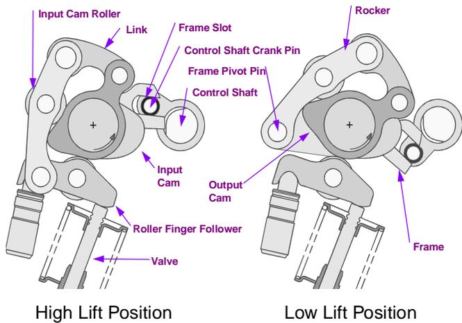
Figure 1. Roller Finger Follower VVA Mechanism
