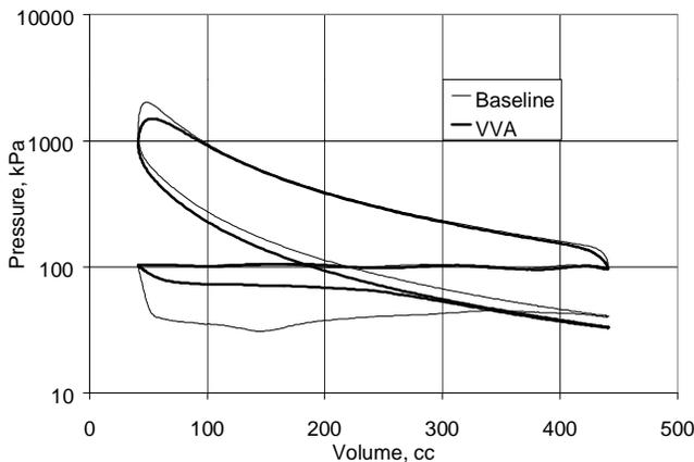
Figure 12. Pressure v. Volume: 2000 rpm / 300 kPa NMEP
