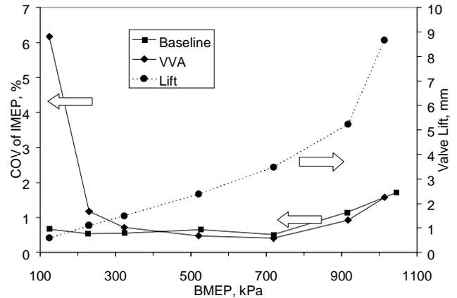
Figure 18. COV of IMEP v. BMEP at 2000 rpm
