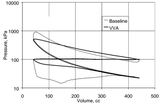
Figure 13. Pressure v. Volume: 2000 rpm / 100 kPa NMEP
