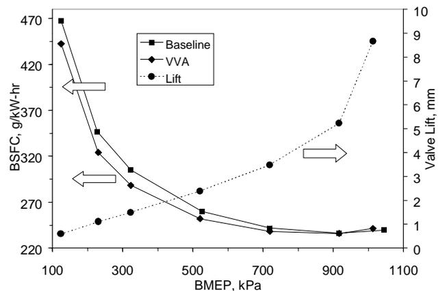
Figure 15. BSFC v. BMEP at 2000 rpm
