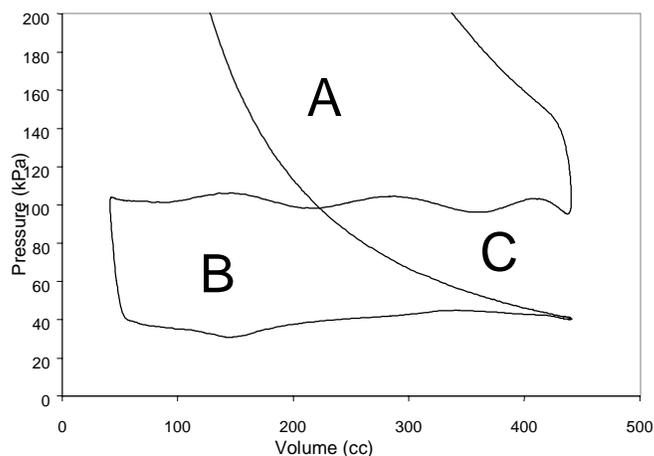
Figure 10. Conventional Engine PV Diagram
