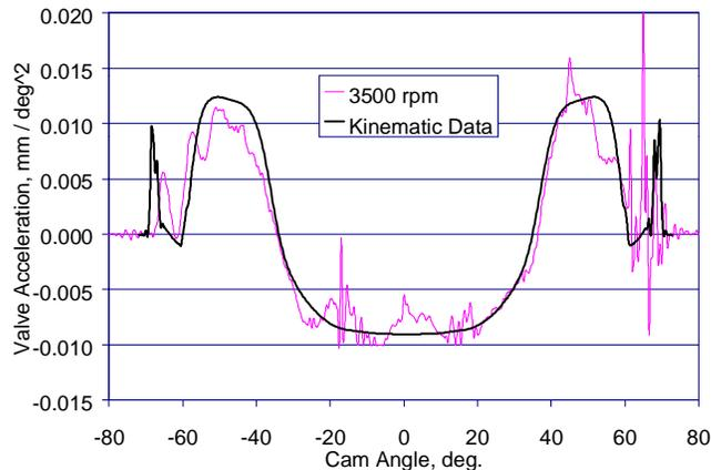
Figure 7. VVA Valve Acceleration at 3500 rpm / 8.9 mm lift
