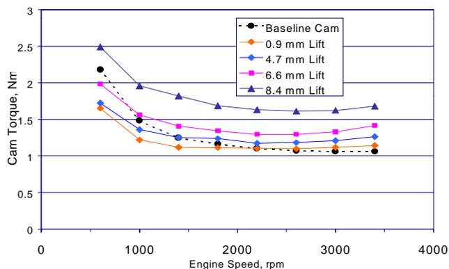
Figure 8. VVA Mechanism Torque
