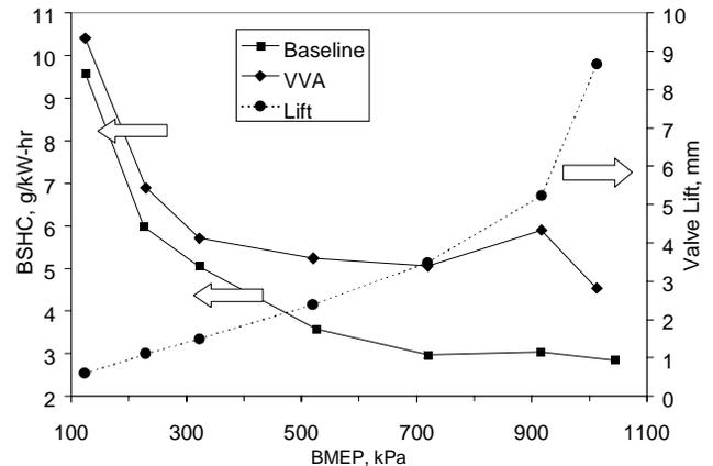
Figure 19. BS HC v. BMEP at 2000 rpm
