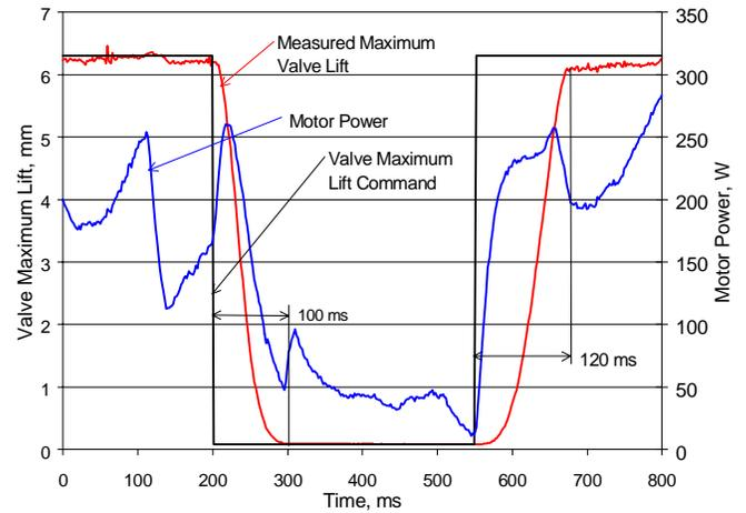
Figure 5. Control System Step Response
