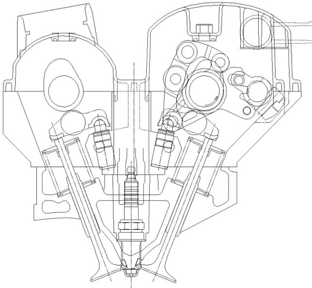
Figure 3. Dynamometer Engine Cross-section
