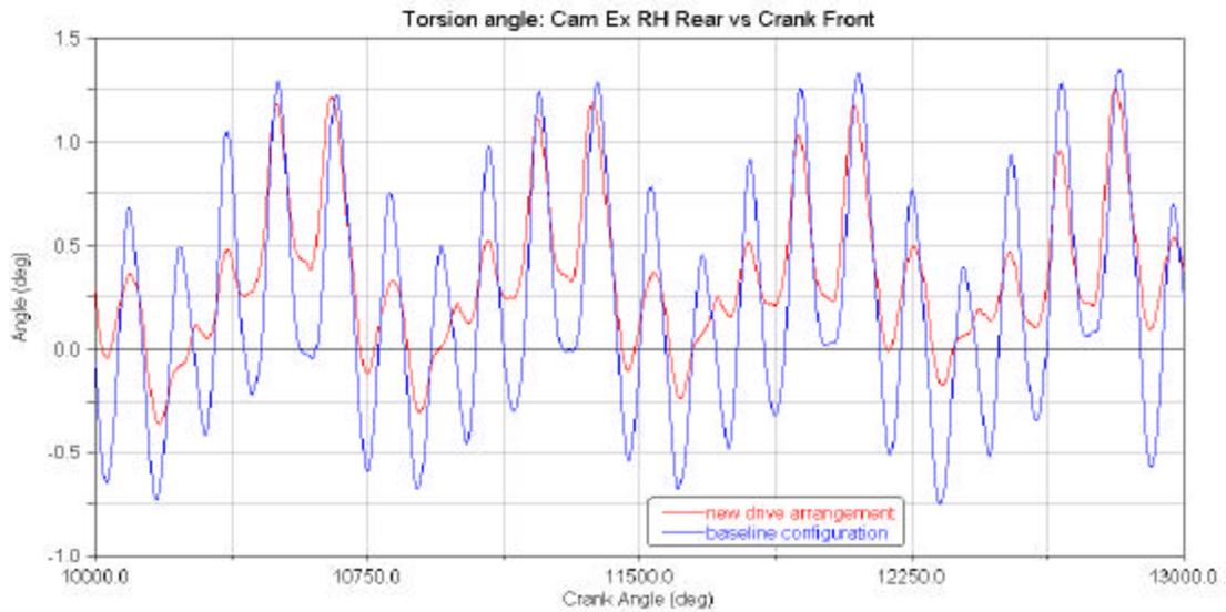
Figure 5. Rear Cam torsion relative to crank front – Cam Ex RH
