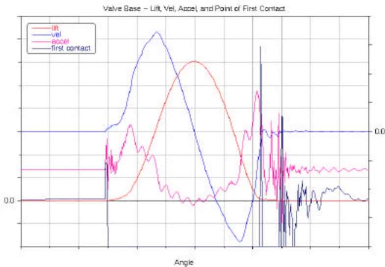
Figure 7. Lift, velocity, acceleration and seat contact force at 9000 cam rpm
