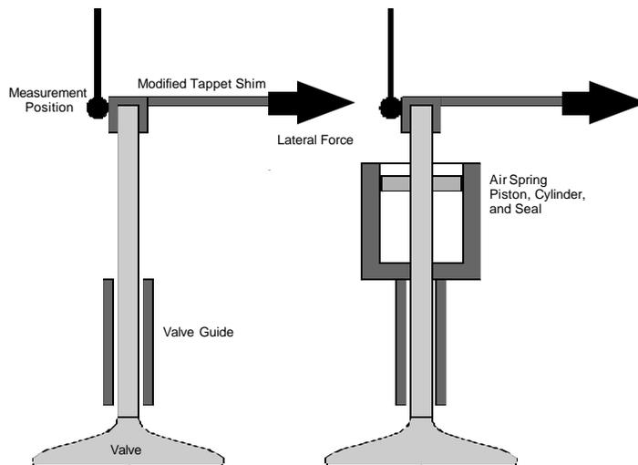
Figure 2. Test configurations for verification of flexible valve model
