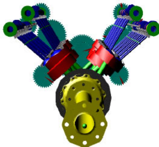
All cams were constrained so that all the valves were on their seats at the start of the analysis. Imposed motions then moved the cams into their required position within the first camshaft revolution (thanks to Christoph for this one). This was required as ADAMS was having difficulty finding static equilibrium when some of the valves were at maximum lift (>15mm worth of movement).
