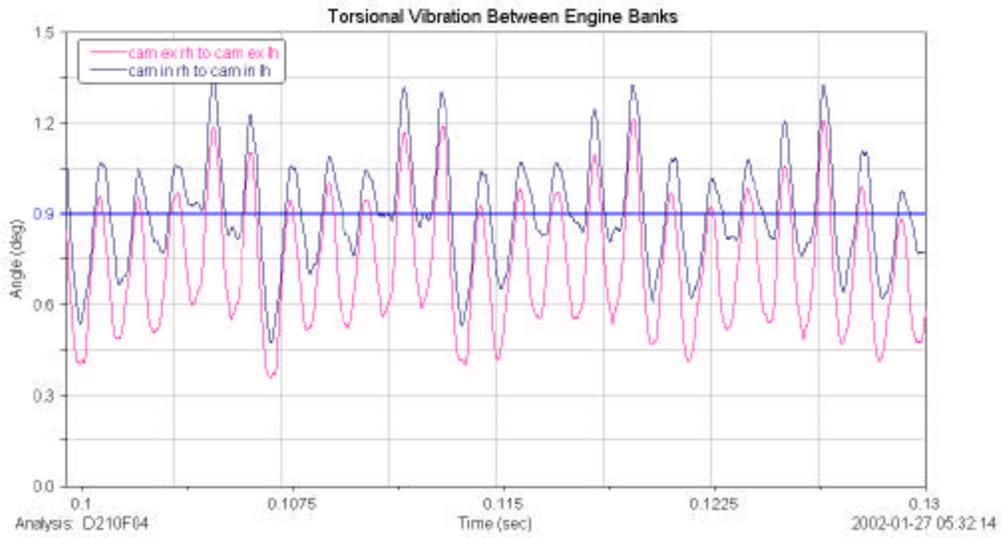
Figure 6. Bank to bank torsional vibration
