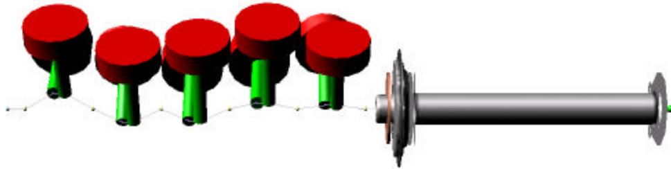
Both the crankshaft and dyno driveshaft were modelled as flex bodies. Previous analyses had shown that crankshaft torsion is sensitive to model detail within the drive arrangement. This model was created before the age of A/Engine Cranktrain, so the valvetrain interface had to be modified to create cranktrain subsystems. Faster run times may now be possible using the FEV beam crank.
