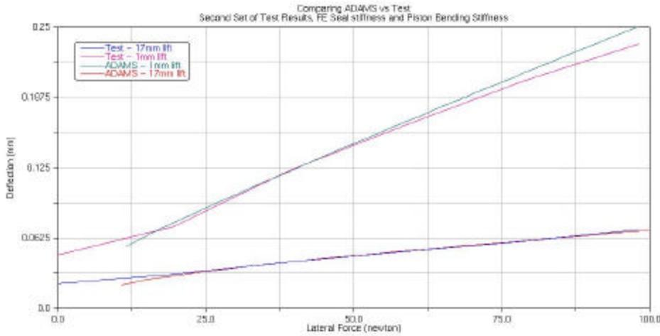
Figure 4. Comparison of valve and air spring lateral stiffness with test
