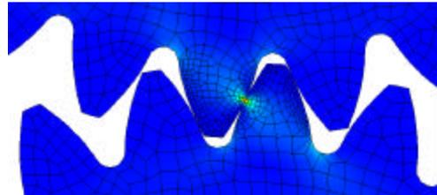
The vibration isolation/compound gears were modelled with a torsional stiffness from mechanical test data. The damping produced by these gears was modelled with stick-slip friction derived again from test data.
