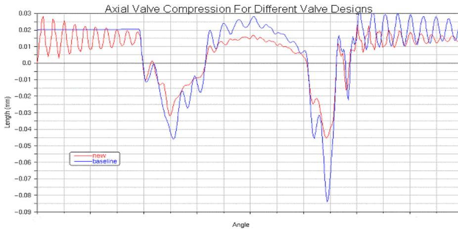
Figure 8. Axial valve deformation – showing improvement in new valve design
