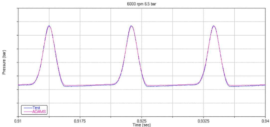
Figure 1. Comparison of air spring model with test
