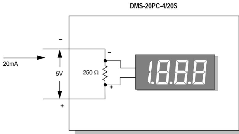
$$\text{Loop Drop} = 250 \Omega \times .020A = 5V$$
