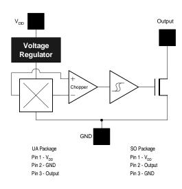
**Note:** This is a static-sensitive device; please observe ESD precautions. Reverse  $V_{DD}$  protection is not included. For reverse voltage protection, a 100R resistor in series with  $V_{DD}$  is recommended.
