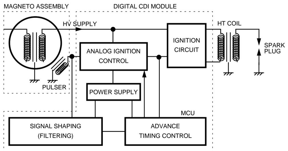
**Figure 4. Typical Digital CDI System Block Diagram**
