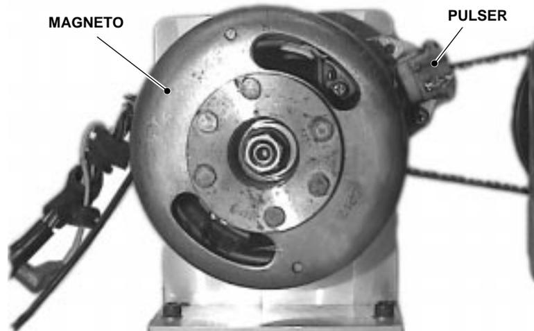
**Figure 1. Magneto/Pulser Assembly**
