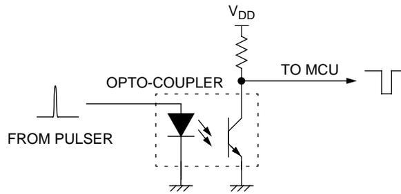
**Figure 7. Pulse Shaping**
