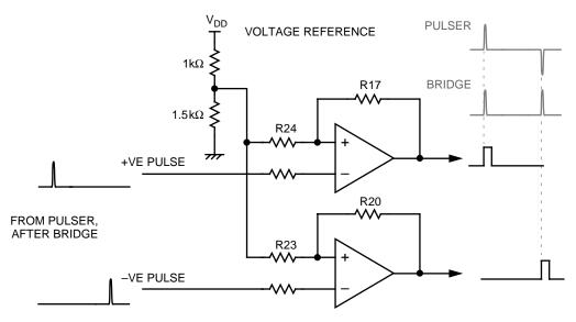
Figure 3. Signal Shaping
