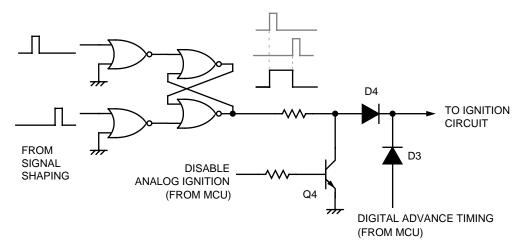
Figure 4. Analog Ignition Control
