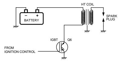
Figure 6. Ignition Circuit
