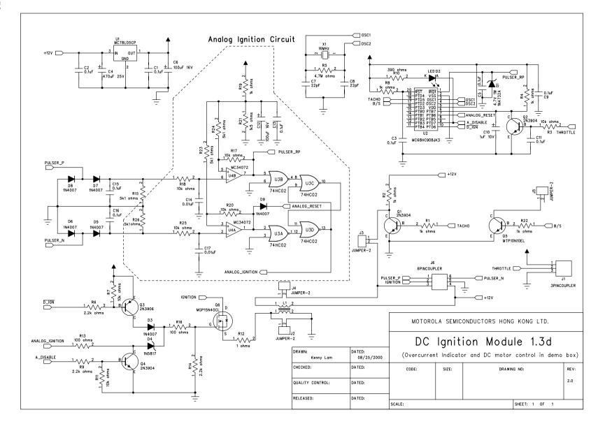
Figure 9. DCI Module Schematics
