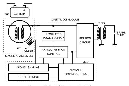
Figure 1. Digital DCI System Block Diagram
