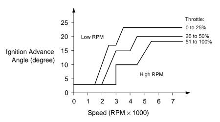
Figure 7. Example of Ignition Advance Characteristics
