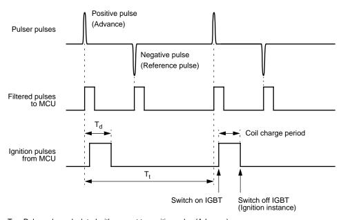
$T_d$  = Delay value calculated with respect to positive pulse (Advance)
