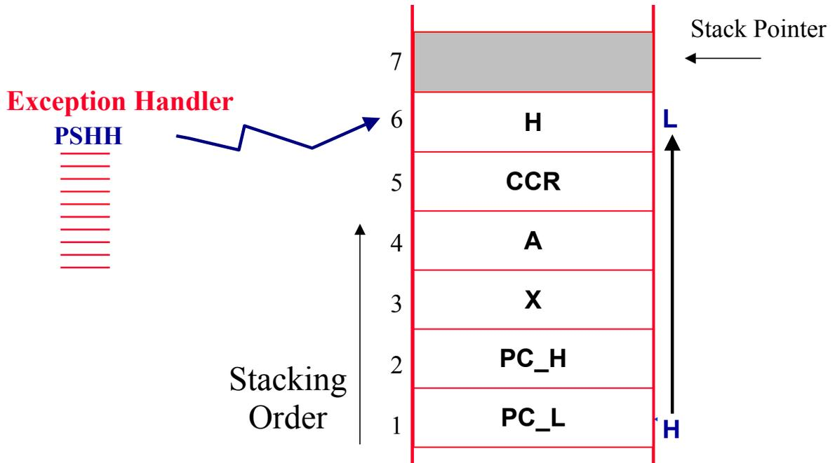
Notice the stacking order of the registers. The registers are stacked from the highest to the lowest address. We mentioned before that the H register is not automatically saved by the CPU. Therefore, it must be saved at the beginning of the exception handler by executing a PSHH instruction. This means that we will have to restore it prior to exiting the exception handler.
