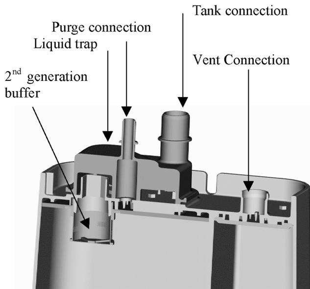
Figure 5. Cross-section of a Delphi ORVR canister (with 2<sup>nd</sup> generation buffer system)
